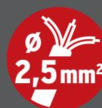
The wire diameter must be selected according to the rated currents. A minimum diameter of  $2.5\text{mm}^2$  is specified for the connection of caravans/motor homes with a rated current of 16A. A smaller wire diameter is not permitted for connecting caravans or motor homes on campsites.
