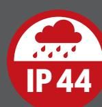
For camping and caravanning use, plugs and couplings as well as sockets must be at least dust and splash-proof (IP44) when plugged in and unplugged.
